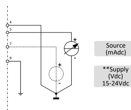
Note: In analog mode with 'mAdc' signals 0Vdc sense (pin 8) does not need to be connected. The instrument's operation will not be effected in case 0Vdc sense is already hooked-up.
