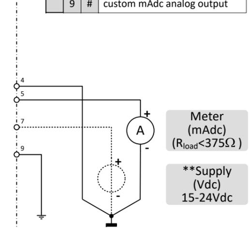
Note: In analog mode with 'mAdc' signals 0Vdc sense (pin 8) does not need to be connected. The instrument's operation will not be effected in case 0Vdc sense is already hooked-up
