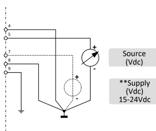
Note: 0Vdc power (pin 4) and 0Vdc sense (pin 8) should be separately connected to the 0V terminal at the power supply.
