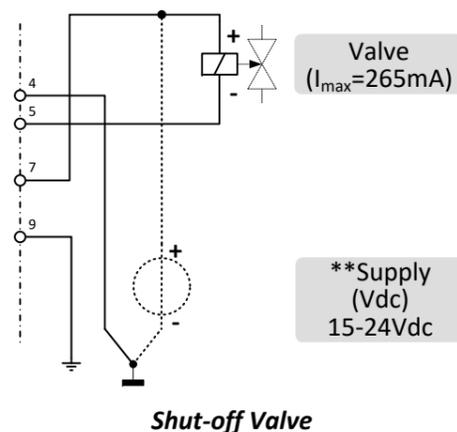
\* Use  $R_{pull-up}$  (between 5k $\Omega$  and 10 k $\Omega$ ) to create 15-24Vdc at pin 5
