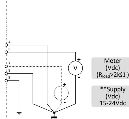
Note: 0Vdc power (pin 4) and 0Vdc sense (pin 8) should be separately connected to the 0Vdc terminal at the power supply
