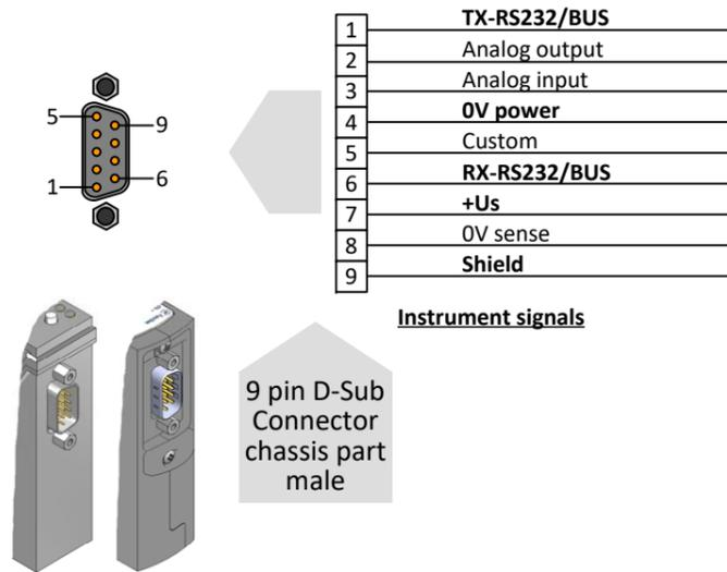
When connecting the system to other devices, be sure that the integrity of the shielding is not affected. Do not use unshielded wire terminals.
