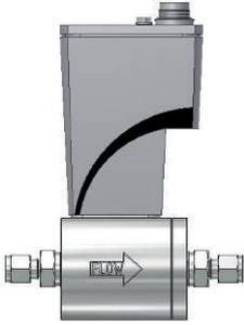
To comply with the IP65 ingress protection standard, the p.c. board is housed in a sealed casted metal housing. For electrical connections the instrument has a 8DIN male connector for analog/RS232 operation and for digital operation various connectors on top. These instruments are suited for light industrial (outdoor) use to IP65.
