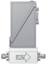
The μ-FLOW model for up to 2 g/h, basically a straight capillary tube with a sensor. For electrical connection the instrument is equipped with a male 9-pin sub D-connector. The instrument is suited for dry (indoor) applications like laboratories.
