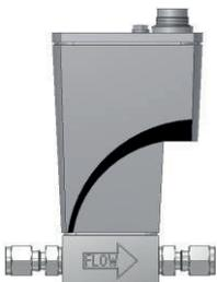
To comply with the IP65 ingress protection standard, the p.c. board is housed in a sealed casted metal housing. For electrical connections the instrument has a 8DIN male connector for analog/RS232 operation and for digital operation various connectors on top. These instruments are suited for light industrial (outdoor) use to IP65.
