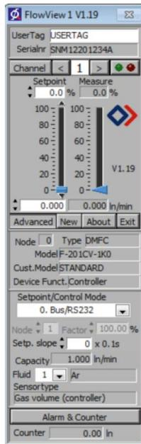
FlowView is an application to easily operate Bronkhorst® digital instruments and readout units (E-8000 series). FlowView is a DDE client and relies on FlowDDE\* for communication to the instruments (standard up to 12 screens, configurable up to 99 screens).
