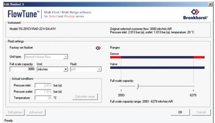
The MFMR functionality is valid for operating conditions from 0.8 to 10 bar abs (up to 100 bar for EL-FLOW Prestige) and 0 to 70°C.
