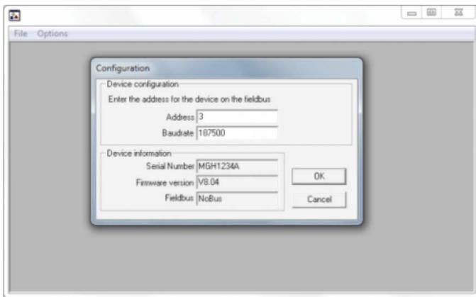
FlowFix is a configuration application for the fieldbus connection and active fluid. It gives an overview of the available fluids (calibration curves) and allows the user to activate the desired fluid, fieldbus address and baudrate.
