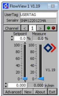
Advanced FlowView window with additional functions: instrument identification, setpoint/control mode, setpoint slope, fluid selection, button for alarm and counter settings, counter value and alarm info.
