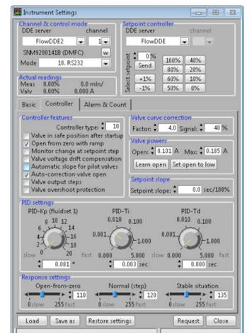
Example of control panel for instrument settings
